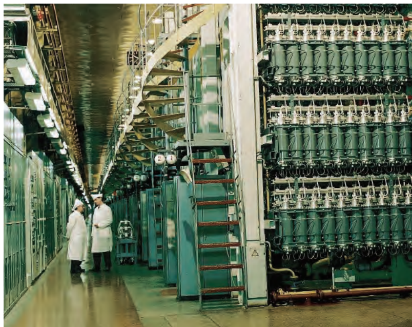
Surprise! Undetected by the U.S. intelligence community, by the mid-1980s the Soviet Union had converted its gaseous-diffusion technology for making highly enriched uranium to the highly efficient gas-centrifuge technology. The centrifuges (shown here) had doubled Soviet production capacity.
