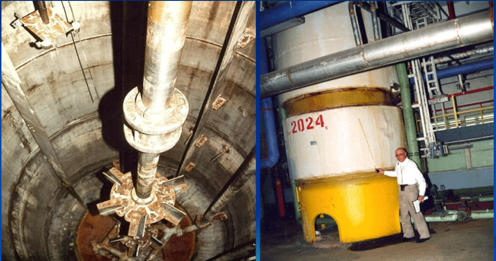
One of ten 20,000-liter fermenters in Russia's Biopreparat's Scientific Experimental and Production Base (SNOPB) Stepnogorsk, Kazakhstan
