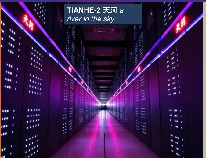
China's 33.68 petaflop Tianhe-2 super computer has 16,000 computer nodes each having two **Intel Ivy Bridge** processors and three Xeon Phi micro-processors. By 2015, the Tianhe-2 is expected to reach 100 petaflops.
